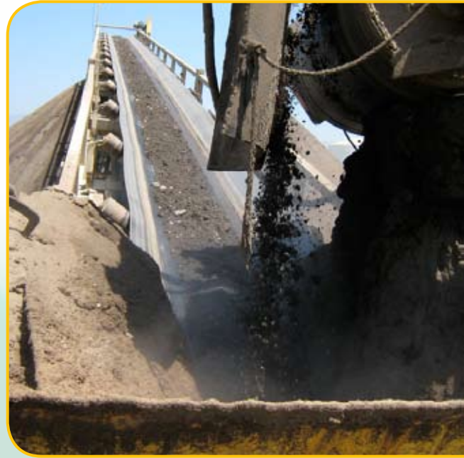
The LTTD produces clean, contaminant-free media at a rate of 30 tons per hour.
